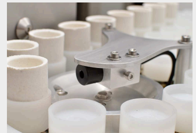
Autoloader with acid-resistant plastic crucible holders
