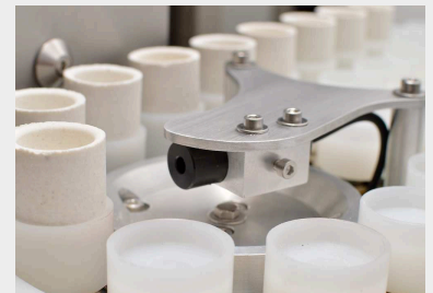
Autoloader with acid-resistant plastic crucible holders
