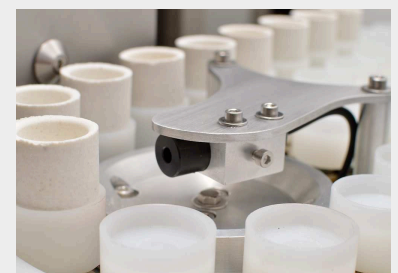
Autoloader with acid-resistant plastic crucible holders
