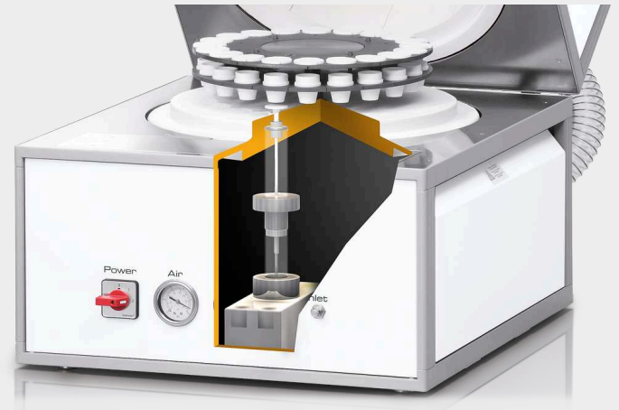
Encapsulated weighing cell
