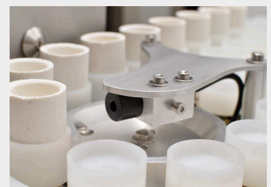
Autoloader with acid-resistant plastic crucible holders
