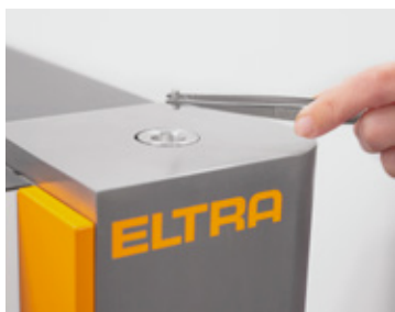
Figure 4: Application of a powdered sample in a nickel capsule
