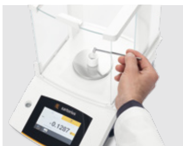
Figure 5: Application of accelerator to a crucible with sample
